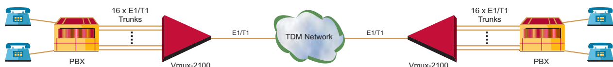
Figure 3. Vmux-2100 Enables Supporting up to 480/384 Voice Channels over a Single E1/T1 TDM Link
