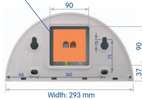
Space for RJ45 wall outlet
